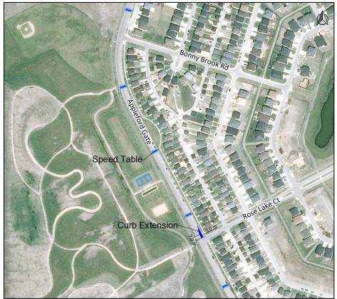
Figure 2: Option 1 – Speed Tables and Curb Extension
