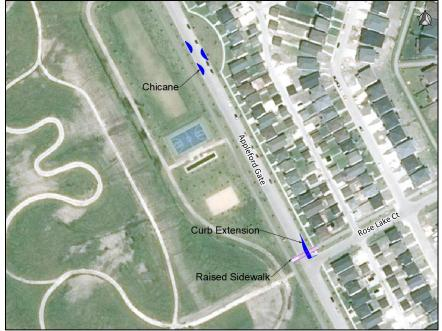
Figure 3: Option 2 – Chicane, Curb Extension, and Raised Crosswalk
