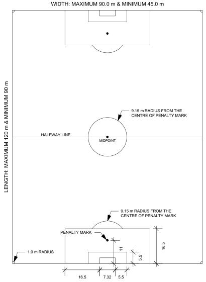
SOCCER FIELD DIMENSION STANDARD ACCORDING TO FIFA SCALE: 1:900
