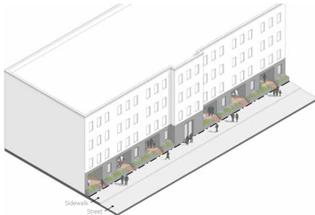
Figure 4 – Embedded Porch Frontage Design Elements
