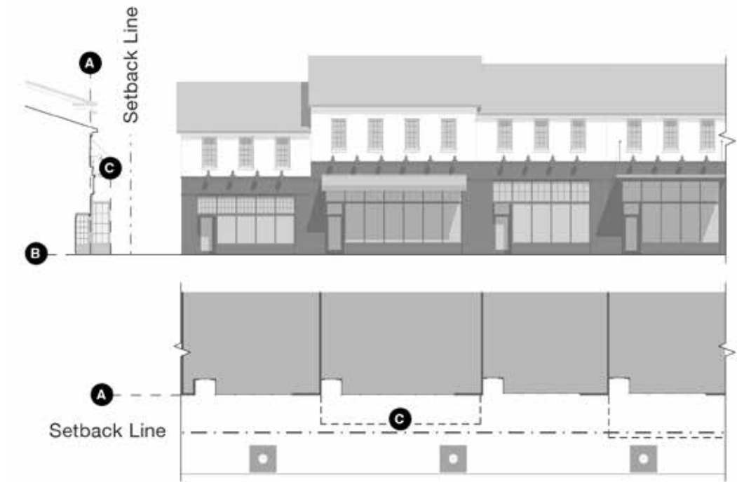
Figure 17 - Illustrated Glazing Requirements
