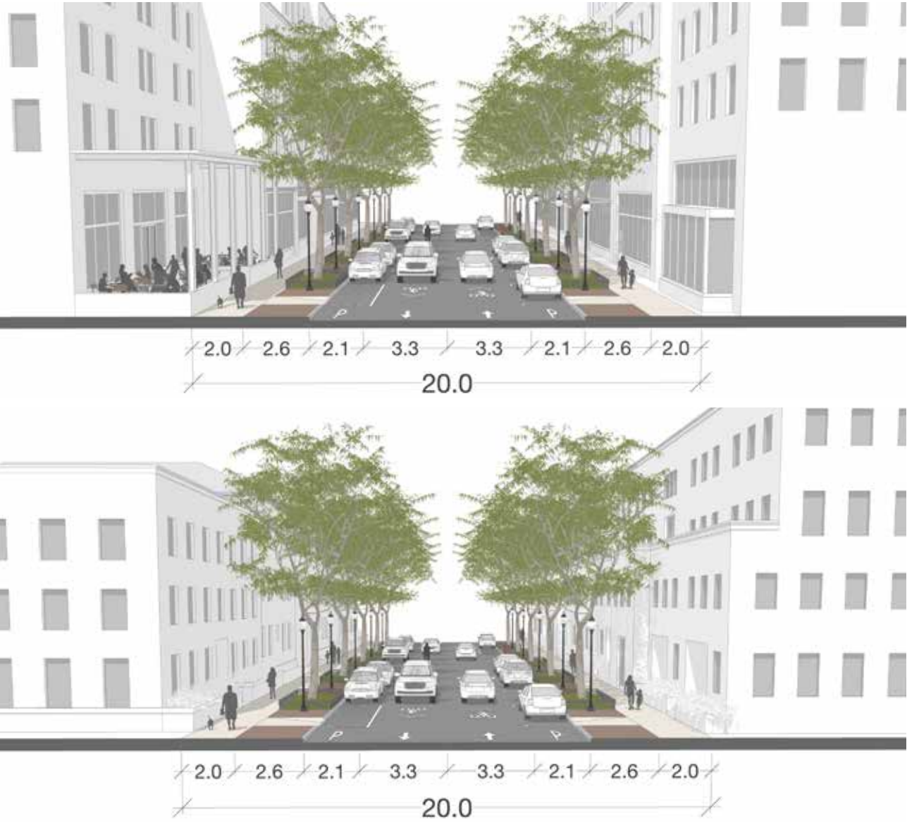
Figure 29 – Typical Framework Street Section
