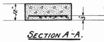
REINFORCING STEEL, MASONRY WALL SLAB.
