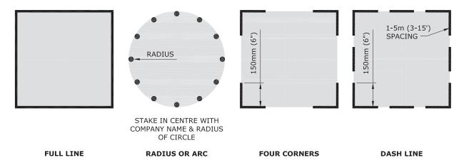
If an excavation is contained within a 5 metre maximum radius then it can be marked with a single white stake at the centre of the excavation. The stake must clearly state the company identifier and the radius of the excavation in black lettering. This information must be conveyed to Manitoba Hydro.
