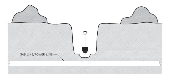
Dig a trench by hand across the full width of the excavation (perpendicular to or "across from" the line). If the line is not uncovered, mechanically excavate to one half the depth of the trench. Repeat this process until the line is exposed.
