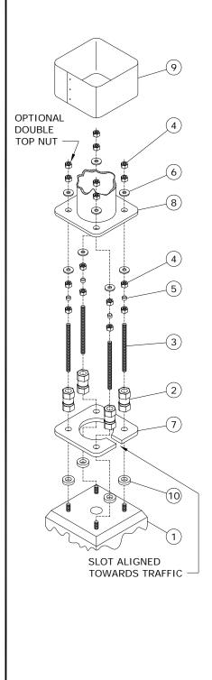
THE FOLLOWING INSTALLATION INSTRUCTIONS ARE APPLICABLE TO NEW OR EXISTING BREAKAWAY BASE INSTALLATIONS ON CONCRETE BASES.
