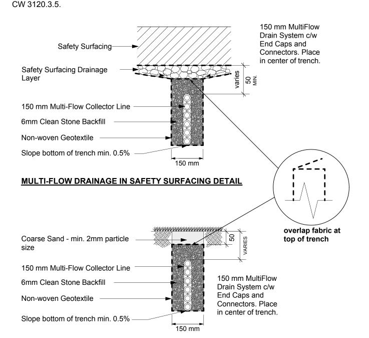
MULTI-FLOW DRAINAGE IN TURF DETAIL
