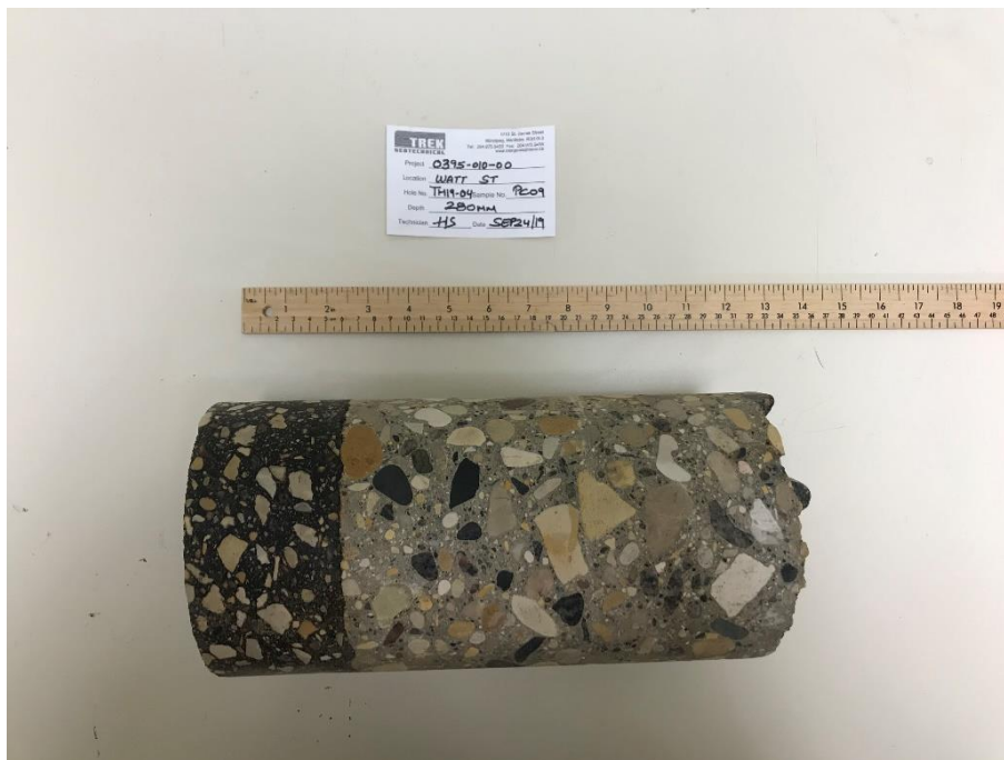
Photo 4: Pavement Core Sample at Test Hole TH19-04
