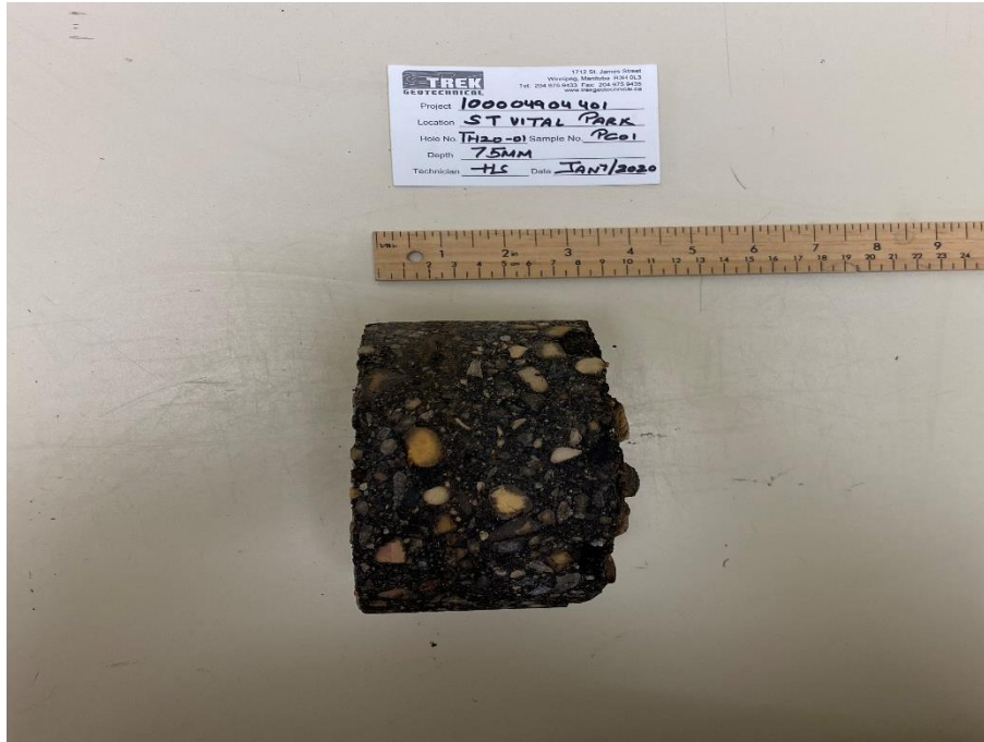
Photo 1: Pavement Core Sample at Test Hole TH20-01
