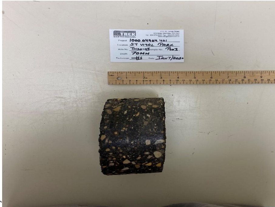
Photo 3: Pavement Core Sample at Test Hole TH20-03
