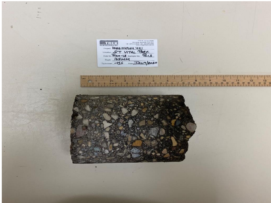
Photo 13: Pavement Core Sample at Test Hole TH20-13
