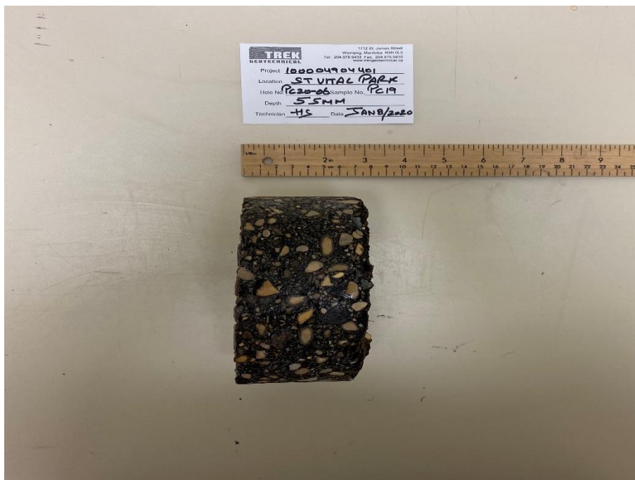
Photo 6: Pavement Core Sample at Pavement Hole PC20-06
