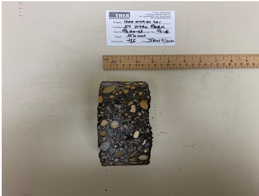
Photo 3: Pavement Core Sample at Pavement Hole PC20-03
