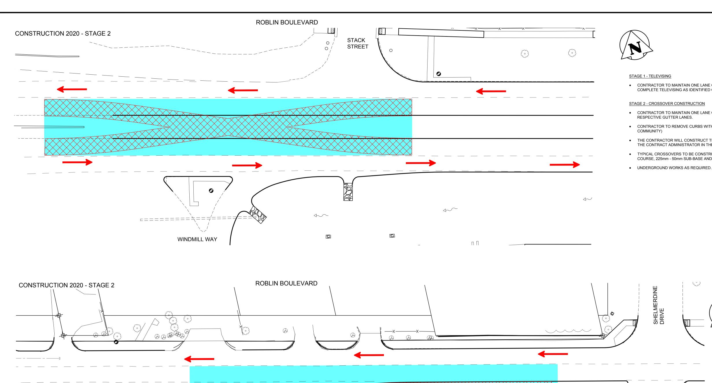
CONTRACTOR TO MAINTAIN ONE LANE OF TRAFFIC IN EACH DIRECTION AS REQUIRED TO COMPLETE TELEVISING AS IDENTIFIED ON THE UNDERGROUND DRAWINGS.
