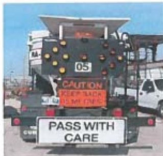
Figure 1.2 and 1.3: Roadpatcher with directional lighting and informational sign (note front and rear mounted beacon lights)
