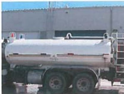
Figure 1.0 and 1.1: Tanker equipped with 4 beacons, retro-reflective striping and combined directional lighting/caution signage.
