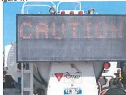
Figure 1.0 and 1.1: Tanker equipped with 4 beacons, retro-reflective striping and combined directional lighting/caution signage.
