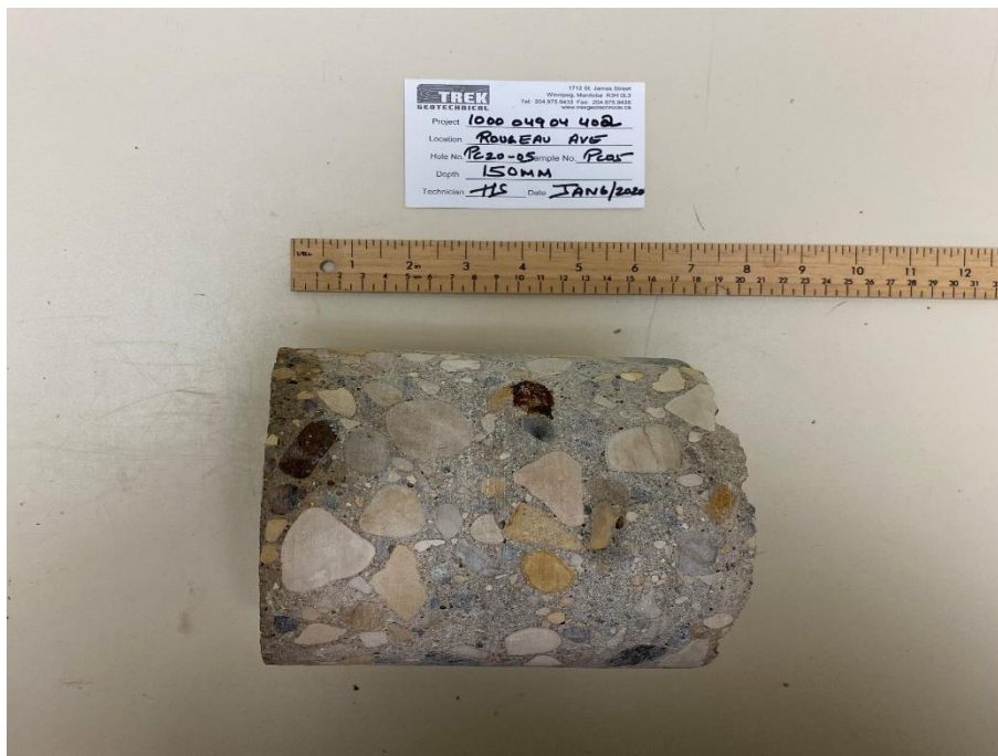
Photo 2: Pavement Core Sample at Pavement Hole PC20-05
