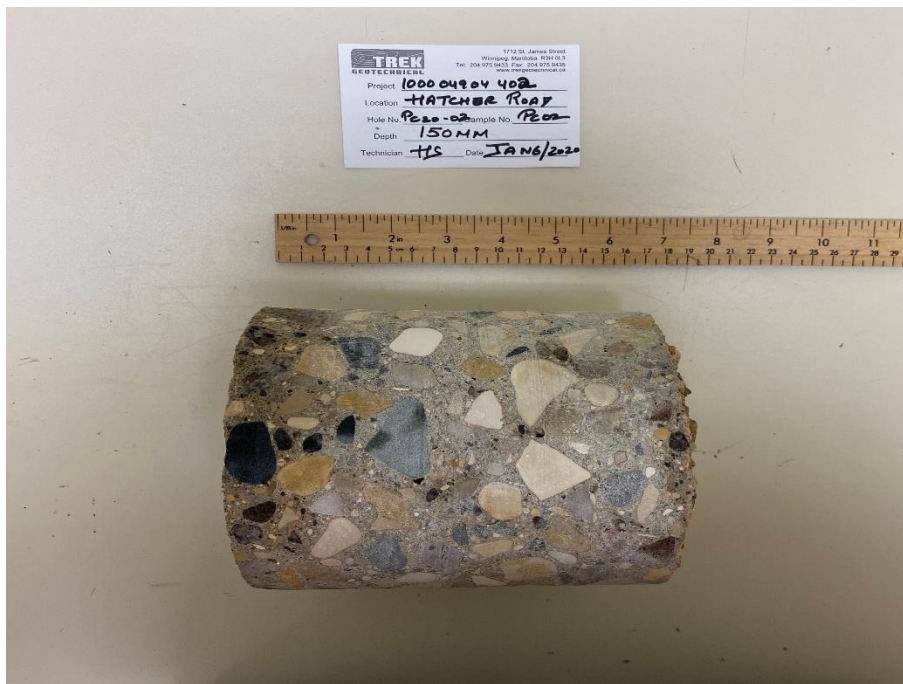
Photo 2: Pavement Core Sample at Pavement Hole PC20-02
