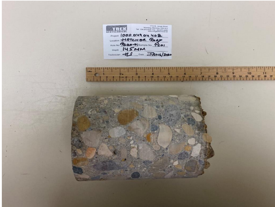
Photo 1: Pavement Core Sample at Pavement Hole PC20-01
