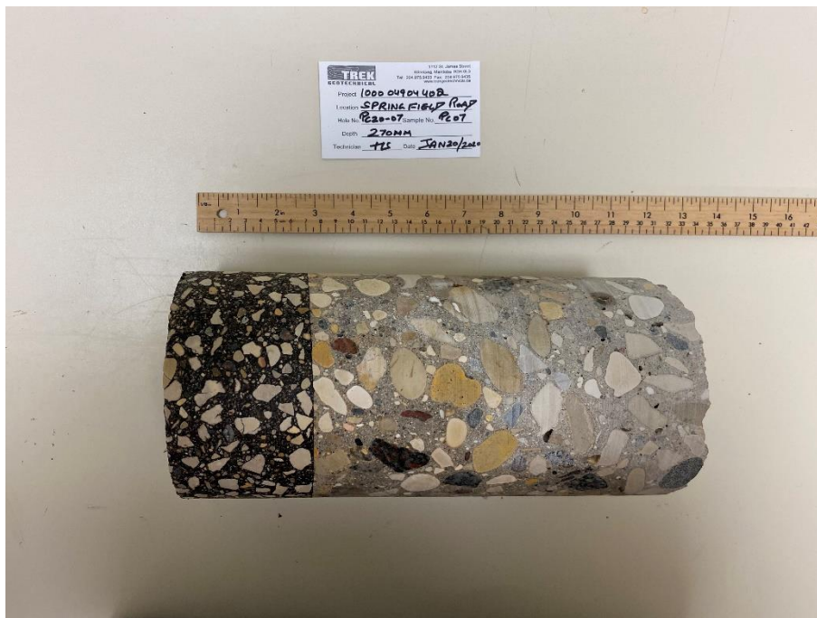
Photo 2: Pavement Core Sample at Pavement Hole PC20-07
