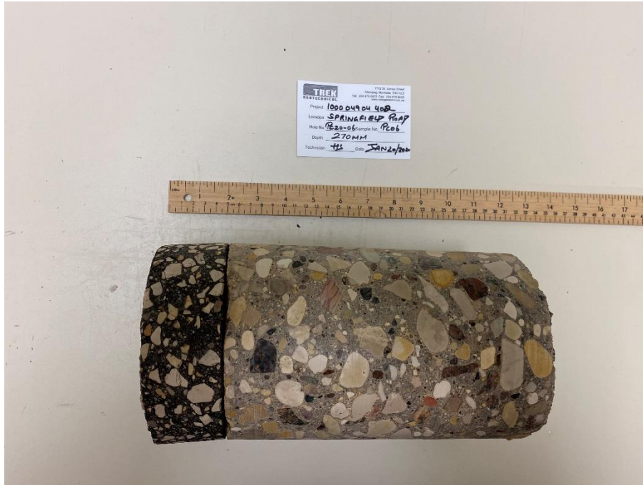
Photo 1: Pavement Core Sample at Pavement Hole PC20-06
