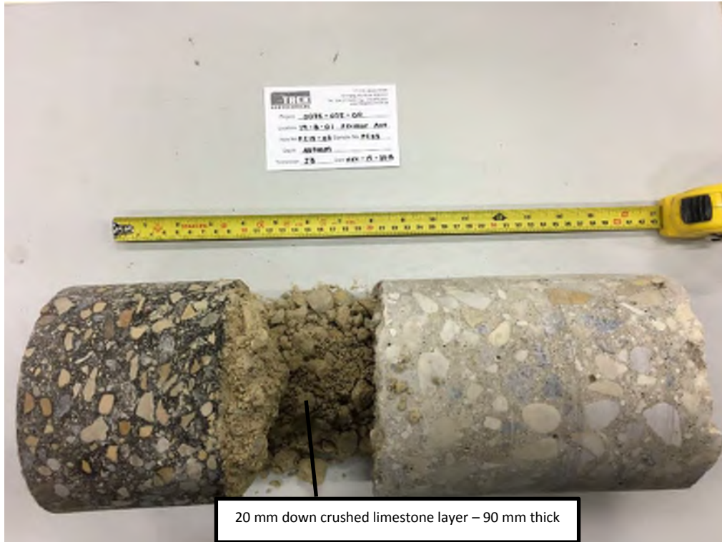
Photo 3: Pavement Core Sample at Test Hole TH18-03
