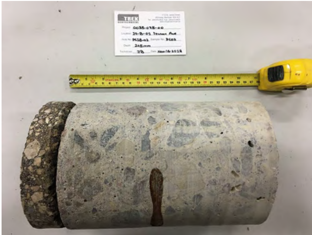
Photo 2: Pavement Core Sample at Test Hole PC18-02
