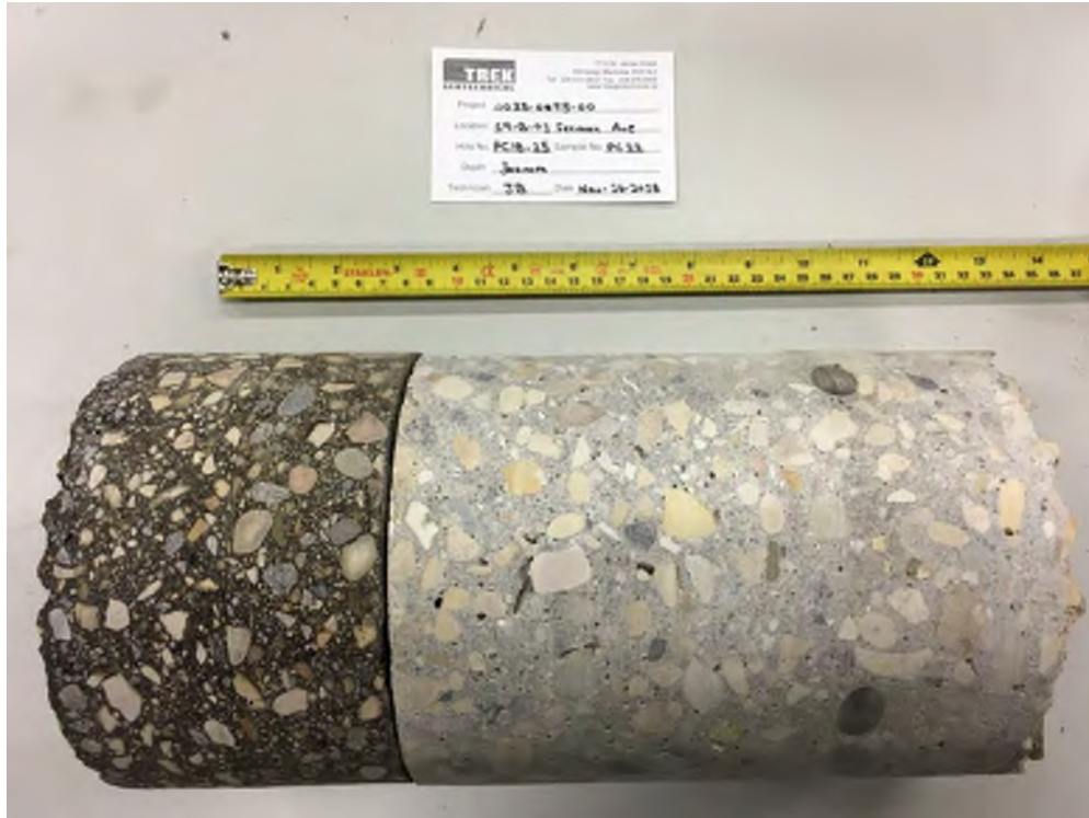
Photo 19: Pavement Core Sample at Test Hole TH18-25
