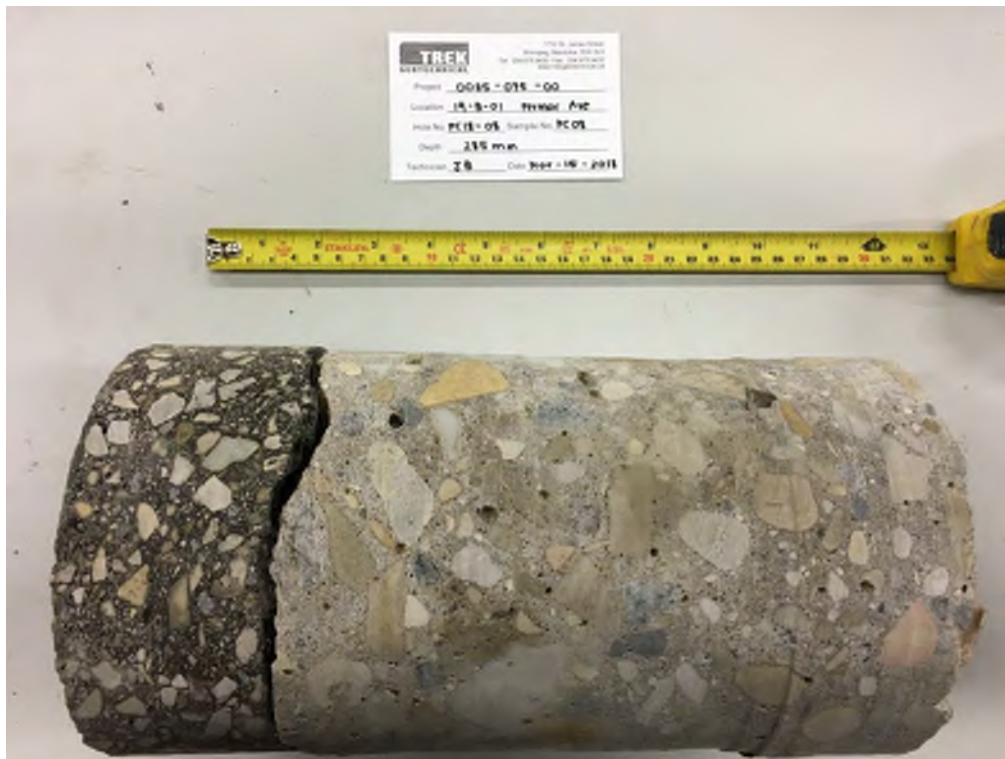
Photo 8: Pavement Core Sample at Test Hole TH18-08
