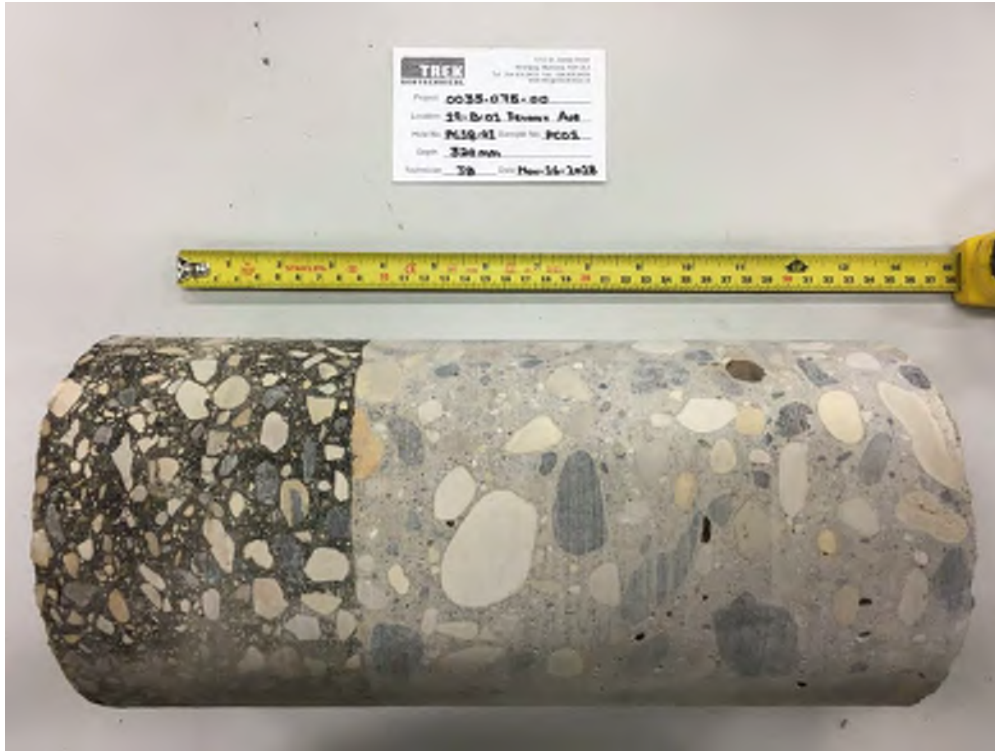
Photo 1: Pavement Core Sample at Test Hole PC18-01
