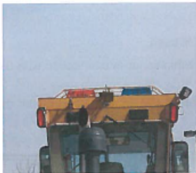
Motor Grader with Dual Rotating Strobe lights, where blue is active only during Winter snow removal
