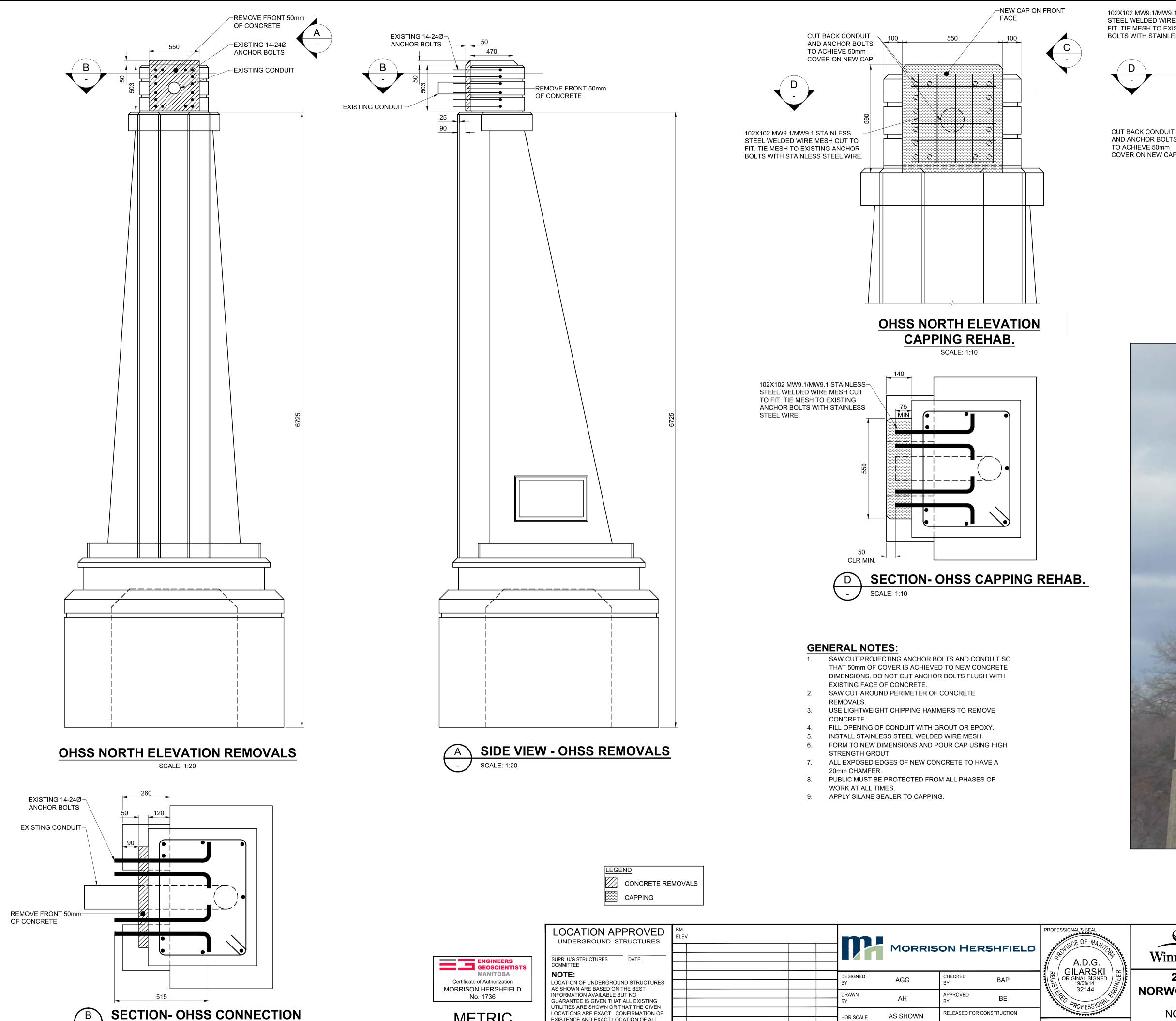
102X102 MW9.1/MW9.1 STAINLESS STEEL WELDED WIRE MESH CUT TO FIT. TIE MESH TO EXISTING ANCHOR BOLTS WITH STAINLESS STEEL WIRE. CUT BACK CONDUIT — AND ANCHOR BOLTS CLR MIN TO ACHIEVE 50mm COVER ON NEW CAP
