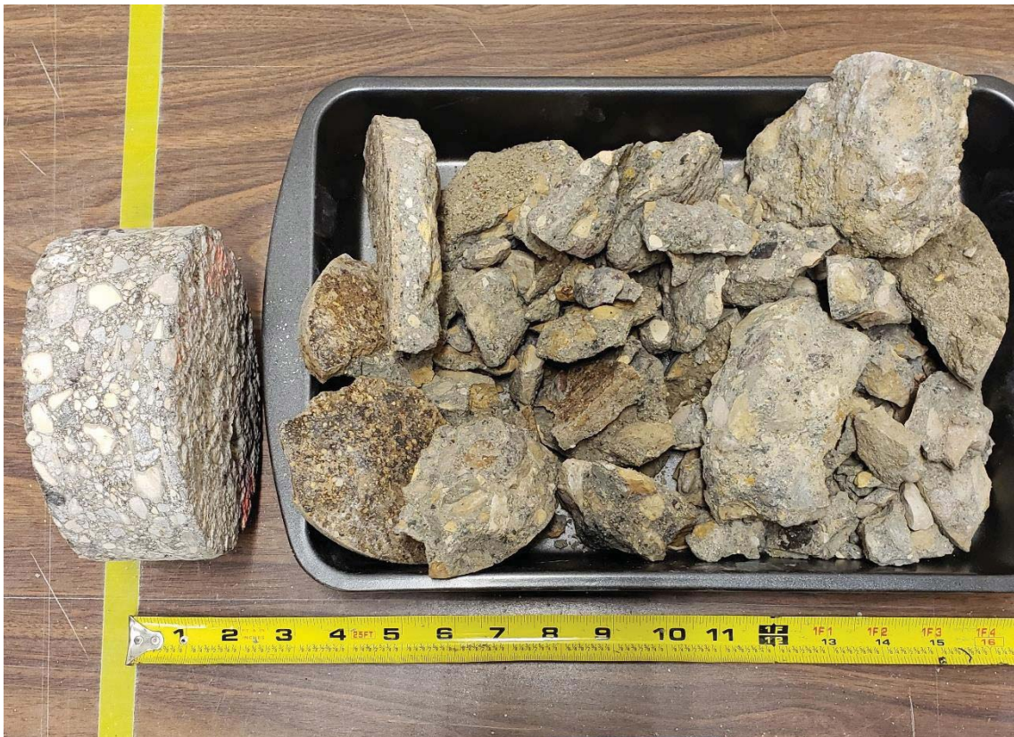
Figure 2 – PC-02 Ainslie St (asphalt and broken concrete, actual core depth 250 mm)
