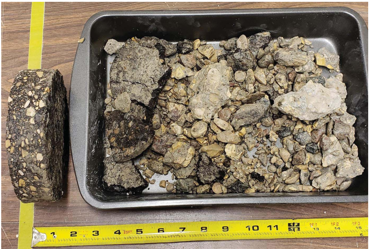
Figure 6 – PC-12 Lodge Ave (asphalt and broken asphalt/concrete, actual core depth 225 mm)
