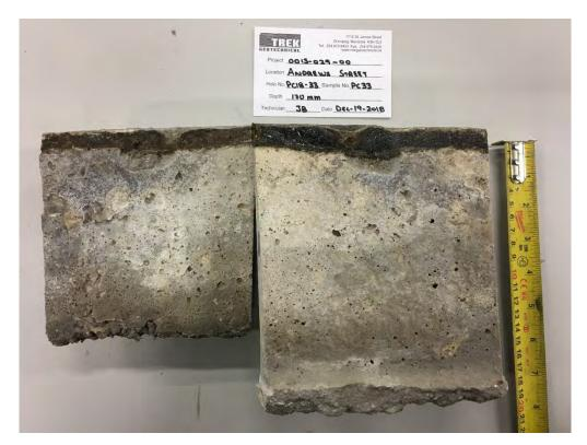
Photo 4: Pavement Core Sample view of Joint at Test Hole PC18-33 Project No. 0015-029-00 January 2019
