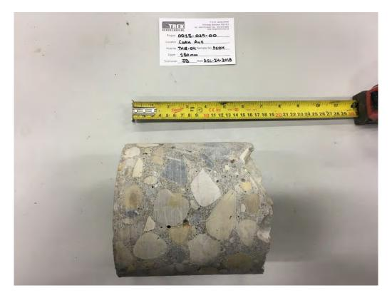
Photo 4: Pavement Core Sample at Test Hole TH18-04 Project No. 0015-029-00 January 2019
