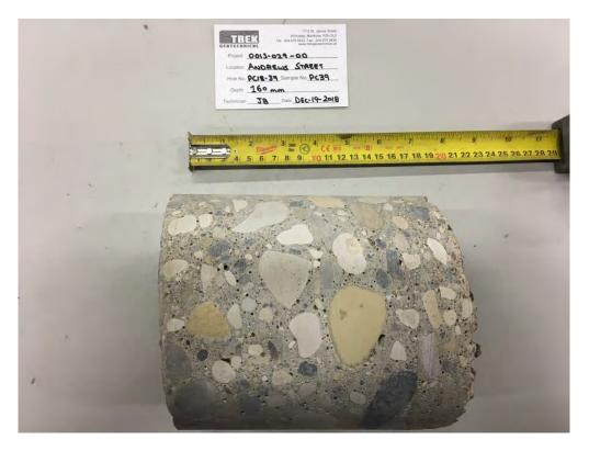
Photo 10: Pavement Core Sample at Test Hole PC18-39
