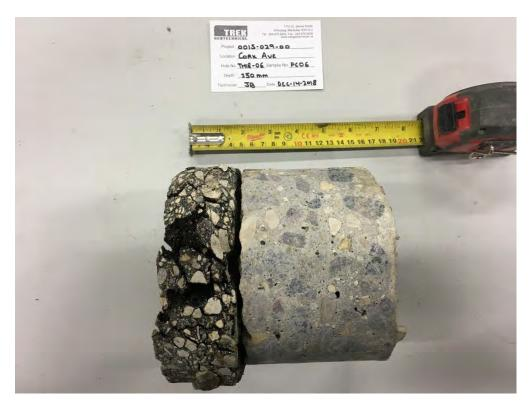
Photo 6: Pavement Core Sample at Test Hole TH18-06
