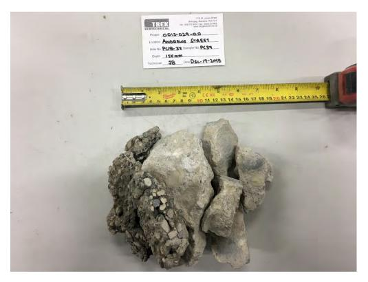
Photo 8: Pavement Core Sample at Test Hole PC18-37
