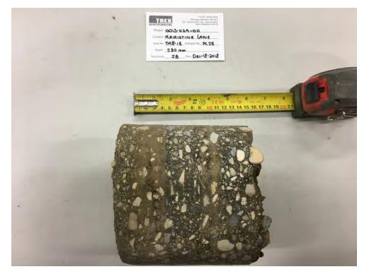
Photo 5: Pavement Core Sample at Test Hole TH18-15
