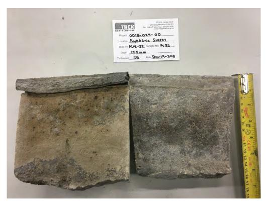
Photo 2: Pavement Core Sample view of Joint at Test Hole PC18-32 Project No. 0015-029-00 January 2019
