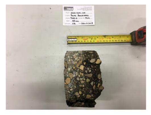
Photo 2: Pavement Core Sample at Test Hole TH18-17
