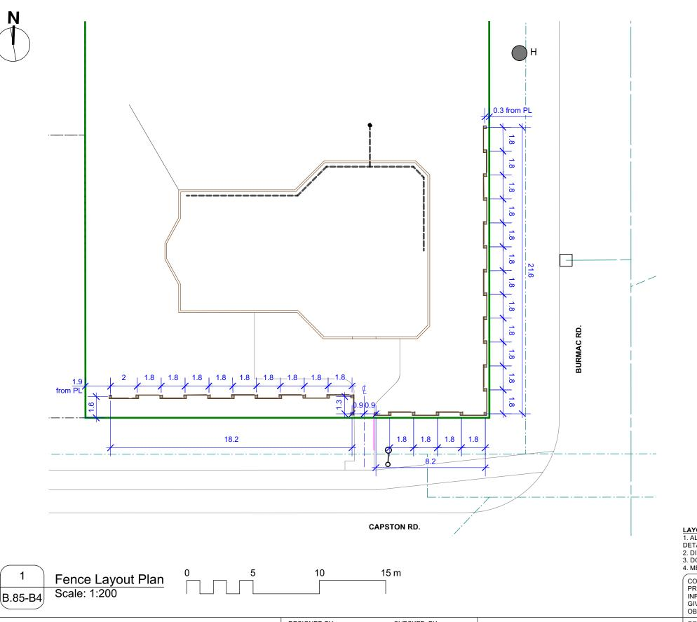
**LEGEND** Park property line Private property line **Existing Water main** Existing hydrant Existing sewer main 0 Existing manhole Existing catch basin  $\bigcirc$ Existing light standard  $\bigcirc$ H Existing hydro pole Existing tree
