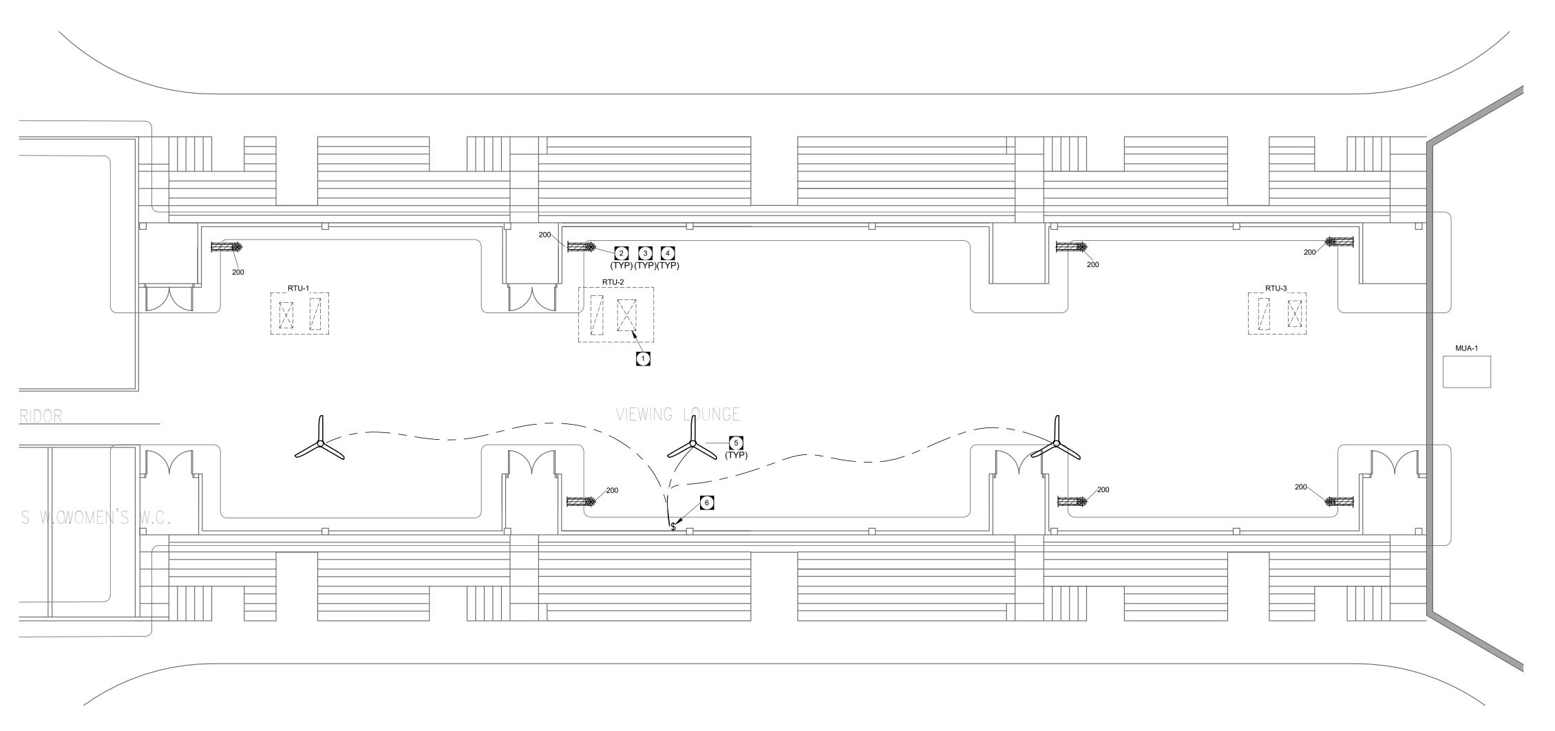
SECOND FLOOR PLAN - HVAC M1 / SCALE: 1:100
