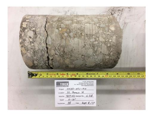
Photo 2: Pavement Core Sample at Test Hole TH17-02
