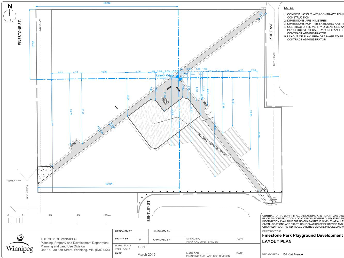
1. CONFIRM LAYOUT WITH CONTRACT ADMINISTRATOR PRIOR TO 2. DIMENSIONS ARE IN METRES 3. DIMENSIONS FOR TIMBER EDGING ARE TO OUTSIDE OF EDGING 4. CONTRACTOR TO VERIFY DIMENSIONS AND CONFORMANCE OF SWING AND PLAY EQUIPMENT SAFETY ZONES AND REPORT ANY DISCREPANCIES TO CONTRACT ADMINISTRATOR 5. LAYOUT OF PLAY AREA DRAINAGE TO BE DETEMINED ON SITE WITH
