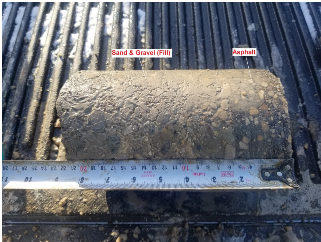
Photograph 8: Test Hole TH19-10 - Hudson Street
