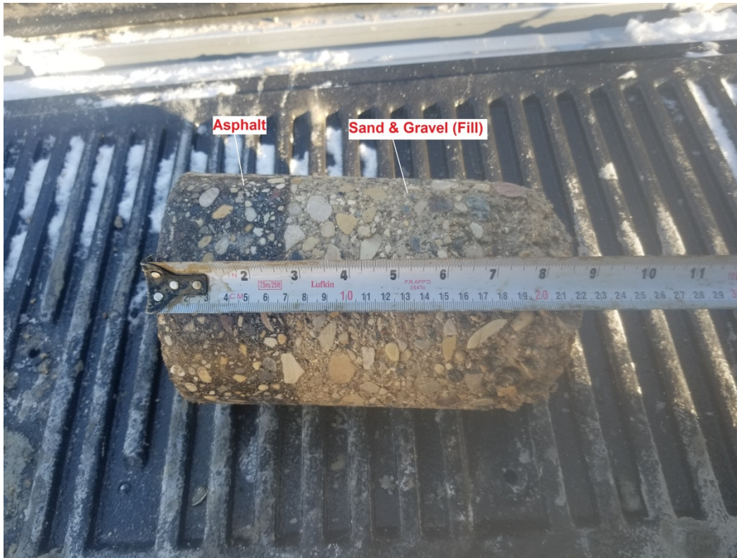
Photograph 11: Test Hole TH19-13 - Hudson Street
