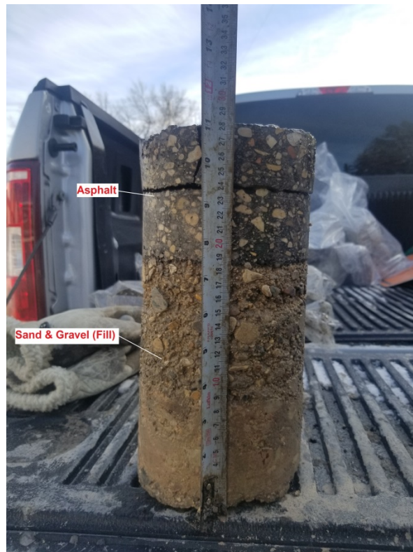
Photograph 12: Test Hole TH19-26 - Villeneuve Boulevard
