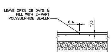
NOTE: SPACING FOR SAW CUTS NOTED ON PLANS OR GENERAL NOTES. FOR AREAS WITH TILE FINISH, PROVIDE SAW CUTS TO MATCH CONTROL JOINTS IN FLOORS
