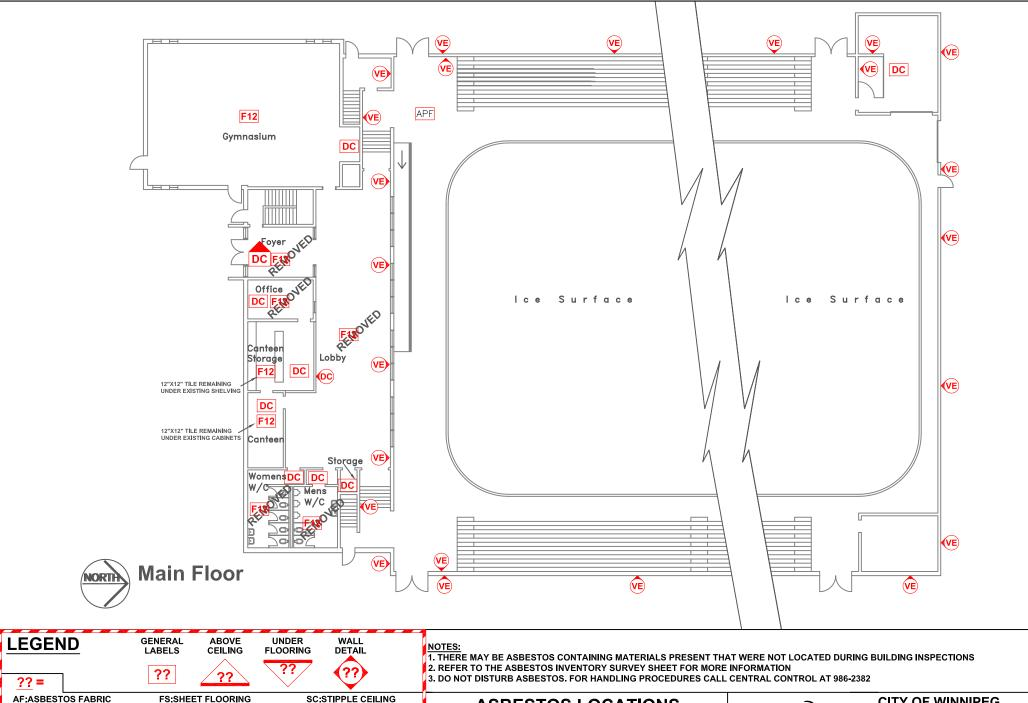
AF: ASBESTOS FABRIC APF: ASPHALT PLANK FLOOR **BR:BOILER REFRACTORY** CA:CAULKING
