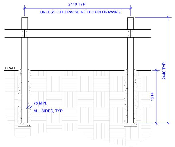
140 x 140 (6" X 6") PT TIMBER POST SLOPE POST TOP, TYP. 38 x 184 (2" X 8") PT TIMBER RAIL. FASTEN W/ 13 (1/2") x 114 (4.5") 200 x 200 (8" X 8") PT TIMBER POST GALVANIZED LAG BOLT & WASHER -SLOPE POST TOP, TYP. PREDRILLED & COUNTERSUNK, TYP. SLOPE CRUSHED LIMESTONE AWAY SLOPE CRUSHED LIMESTONE AWAY 600 FROM POST FROM POST GRADE AGATE PARK SIDE 19 (3/4") CRUSHED LIMESTONE 19 (3/4") CRUSHED LIMESTONE 50 MIN. ALL SIDES TYP.
