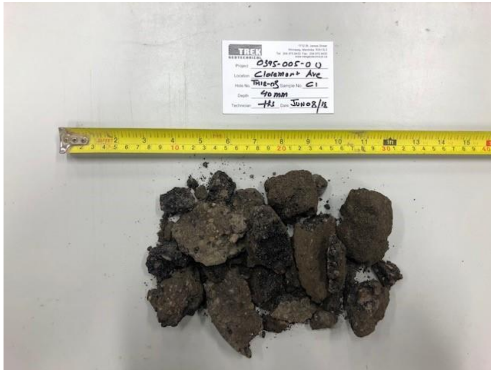
Photo 1: Pavement Core Sample at Test Hole TH18-03
