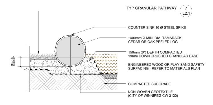
LOG RETAINING WALL DETAIL
