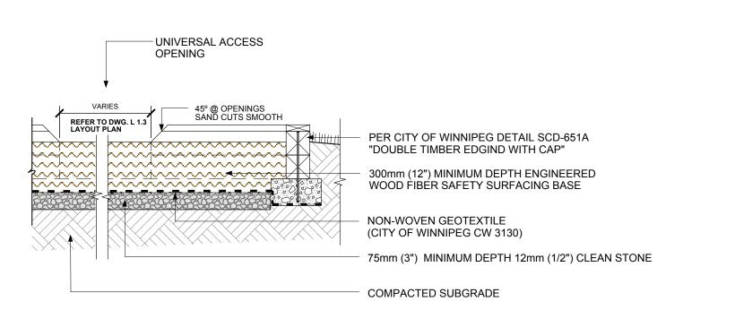
1 SAFETY SURFACING & WOOD TIMBER EDGE DETAIL
