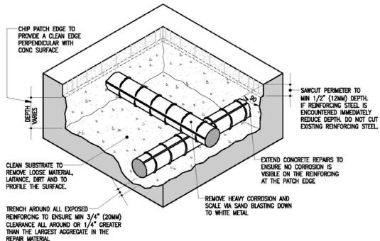
Figure 1: Surface Preparation for Concrete Delamination Repair
