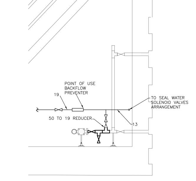
WATER SUPPLY CONNECTION FOR DP LEVEL MEASUREMENT SYSTEM
