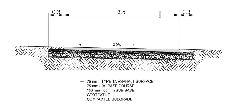
ASPHALT PATH TYPICAL CROSS SECTION
