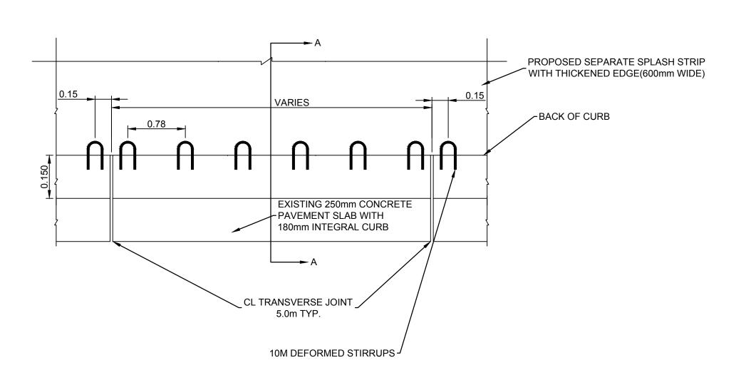
SEPARATE SPLASH STRIP W/ THICKENED EDGE PLAN VIEW **SCALE 1:500**
