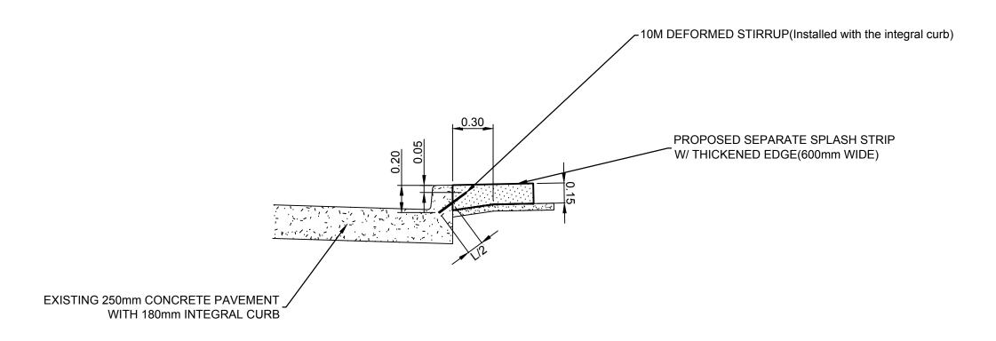
SEPARATE SPLASH STRIP W/ THICKENED EDGE SECTION A - A SCALE 1:20
