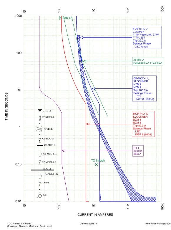
Figure 4-5 - Clifton Lift Pump – Phase 1 TCC Curve
