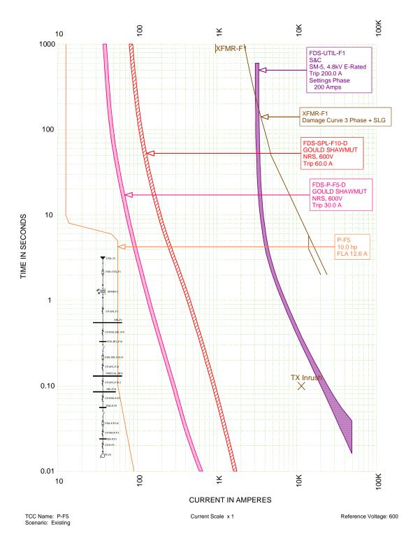
Figure 4-2 - Clifton Pumpout Pump P-F5– Existing TCC Curve
