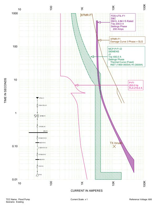
Figure 4-1 - Clifton Flood Pump – Existing TCC Curve
