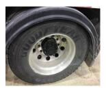
Required: Black rubber, no-name, front and rear of back tires complete with antisail bracket on each mud-flap. Rear mud flaps shall not contact the ground when the dump body is at maximum dump angle
