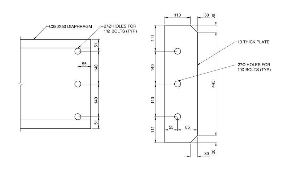
DETAIL - DIAPHRAGM TO GIRDER CONNECTION
