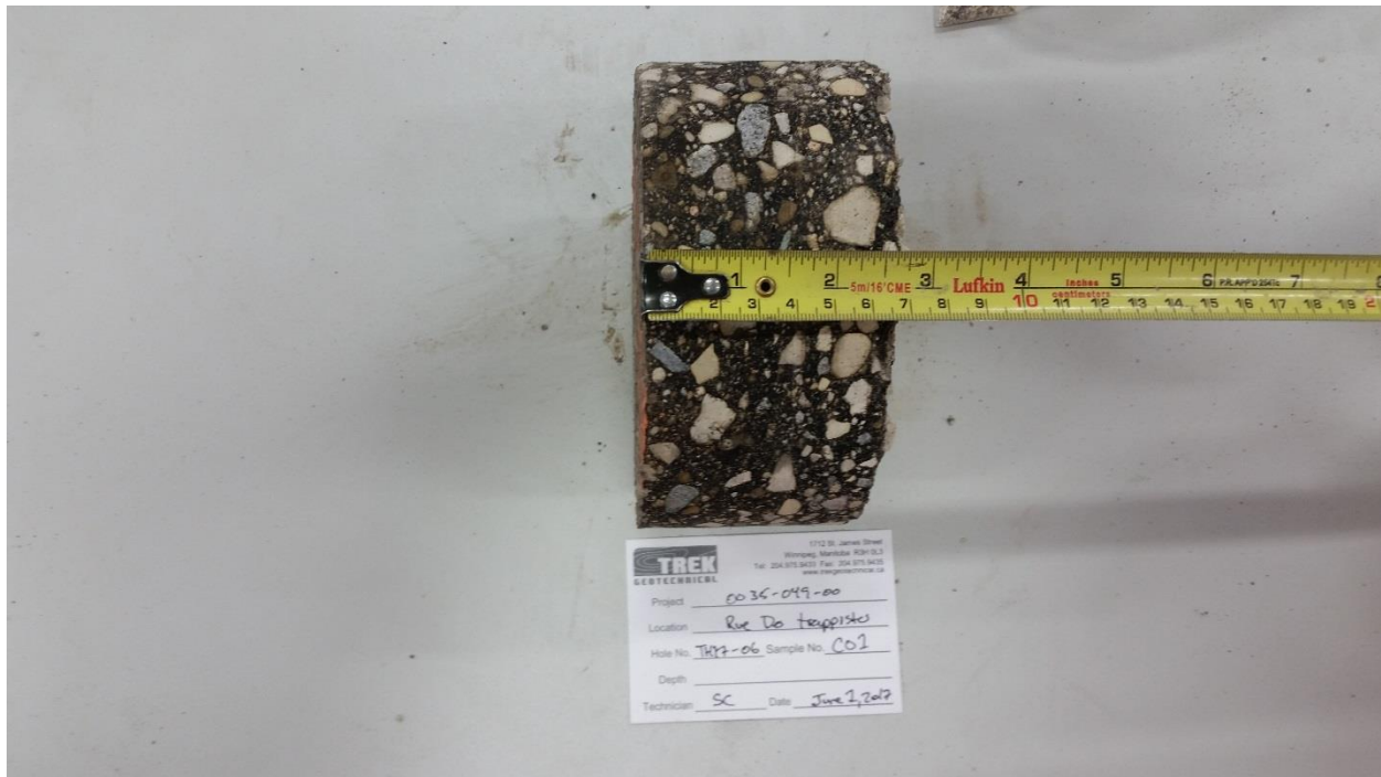
Photo 6: Pavement Core Sample at Test Hole TH17-06
