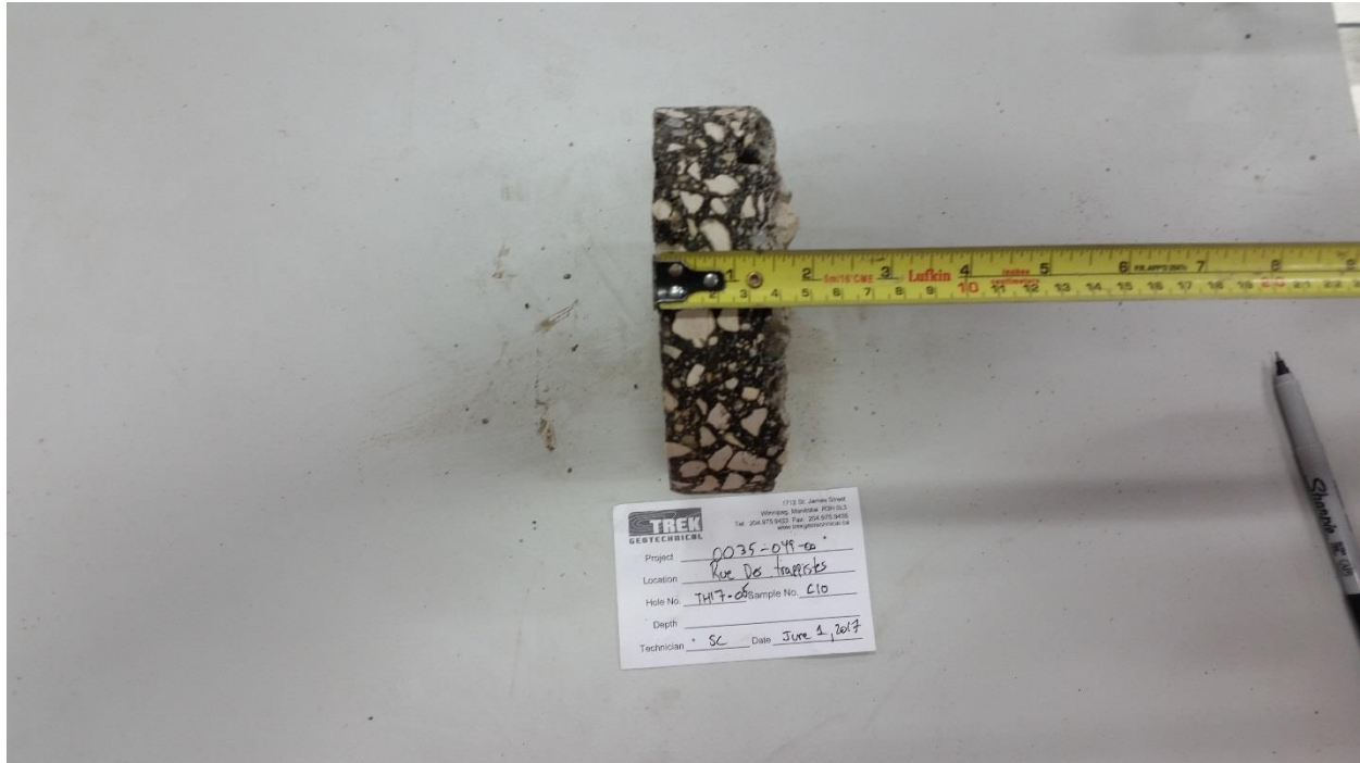
Photo 5: Pavement Core Sample at Test Hole TH17-05
