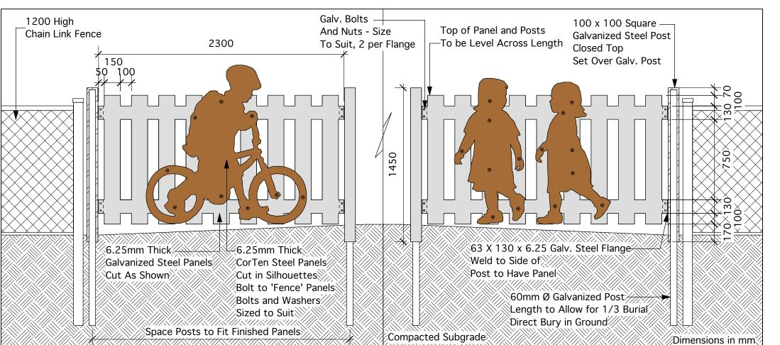
**METAL PANELS - FRONT ENTRANCE** ∖L-6*/* 1:25 150 Dimensions in mm Refer to 2/L-6 for \_Top of Panel and Posts Post, Panel and To be Level Across Length **Fastener Details** 150 R 2\150 200 1450 Concrete Sidewalk
