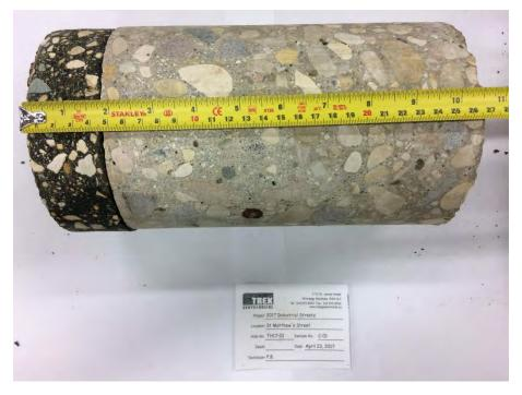
Photo 1: Pavement Core Sample at Test Hole TH17-01
