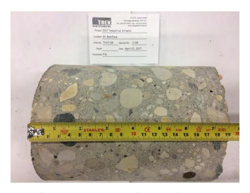
Photo 8: Pavement Core Sample at Test Hole TH17-08
