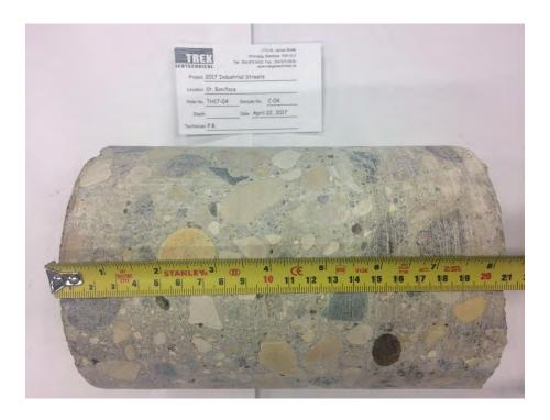
Photo 4: Pavement Core Sample at Test Hole TH17-04
