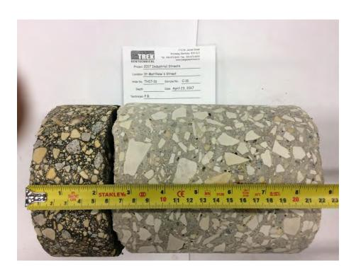
Photo 16: Pavement Core Sample at Test Hole TH17-16
