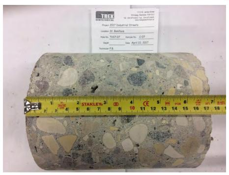
Photo 7: Pavement Core Sample at Test Hole TH17-07
