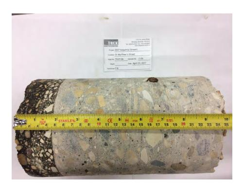
Photo 6: Pavement Core Sample at Test Hole TH17-06
