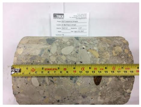
Photo 17: Pavement Core Sample at Test Hole TH17-17
