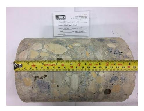
Photo 9: Pavement Core Sample at Test Hole TH17-09
