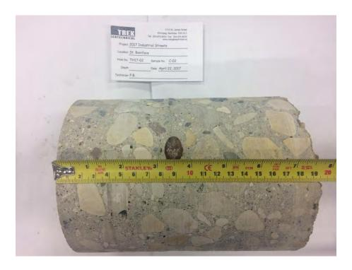
Photo 2: Pavement Core Sample at Test Hole TH17-02
