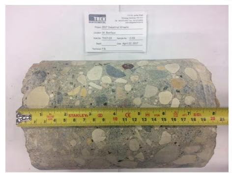
Photo 3: Pavement Core Sample at Test Hole TH17-03
