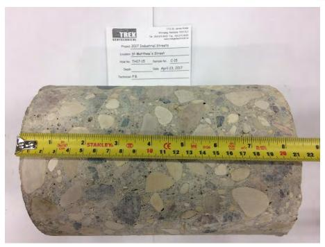
Photo 15: Pavement Core Sample at Test Hole TH17-15
