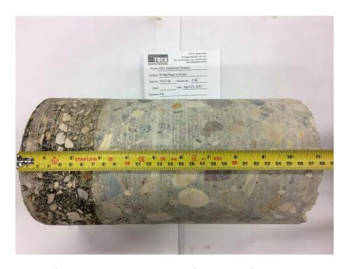
Photo 18: Pavement Core Sample at Test Hole TH17-18
