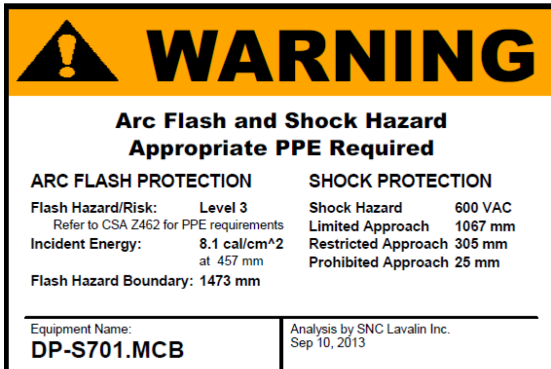
Figure 13-2 : Arc Flash Warning Label, Category 0 through 4 - Large
