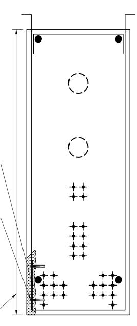
102 X 102 MW9.1/MW9.1 STAINLESS STEEL WELDED-WIRE MESH CUT TO FIT REPAIR AREA, PLACED AT MID-THICKNESS OF PATCH REPAIR. TIE MESH TO EXISTING REINFORCEMENT OR THREADED ROD ANCHORS WITH STAINLESS STEEL WIRE.
