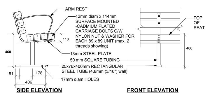
DIMENSIONS SHOWN ARE IN MILLIMETRES UNLESS OTHERWISE SPECIFIED
