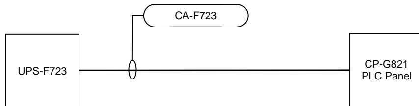
Figure 7-2: Instrument Cable Identification Example – Identified Equipment
