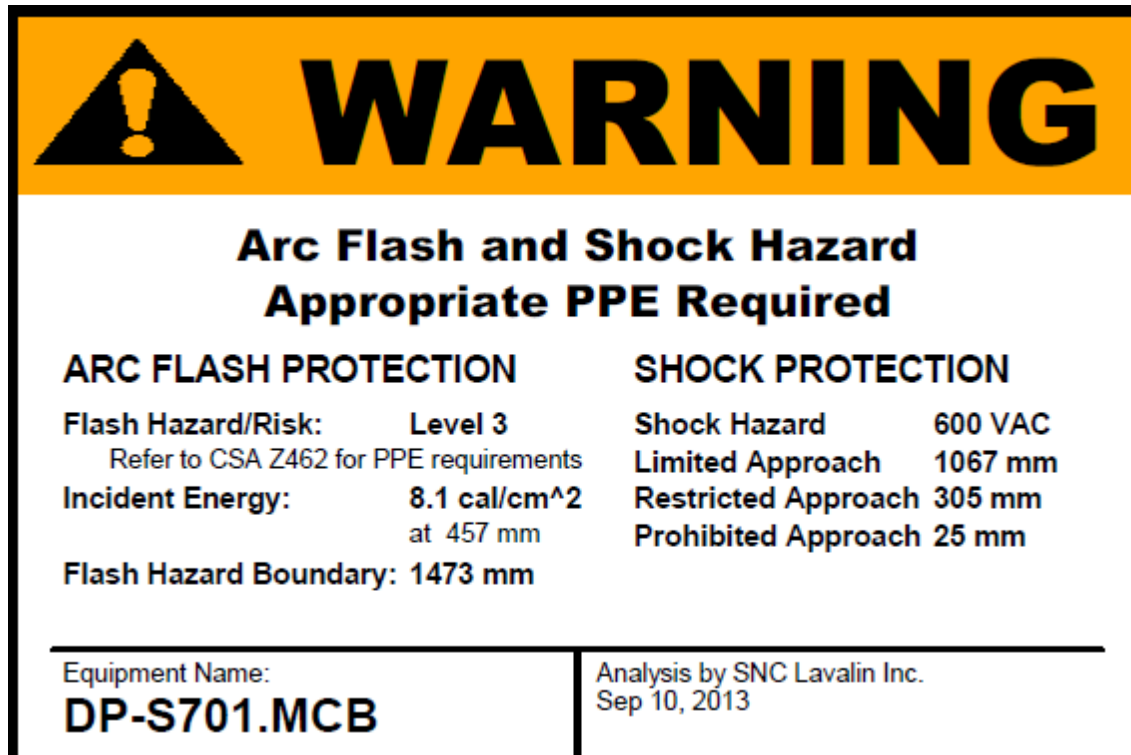
Figure 12-2 : Arc Flash Warning Label, Category 0 through 4 - Large
