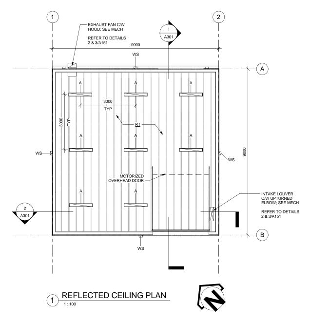
LIGHT FIXTURE SCHEDULE (SEE ELEC): A - EXTERIOR / DAMP RATED LINEAR FIXTURE
