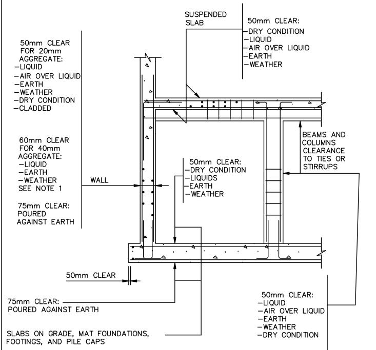
. PROVIDE 50mm CLEARANCE ON FACE EXPOSED TO DRYCONDITION.
