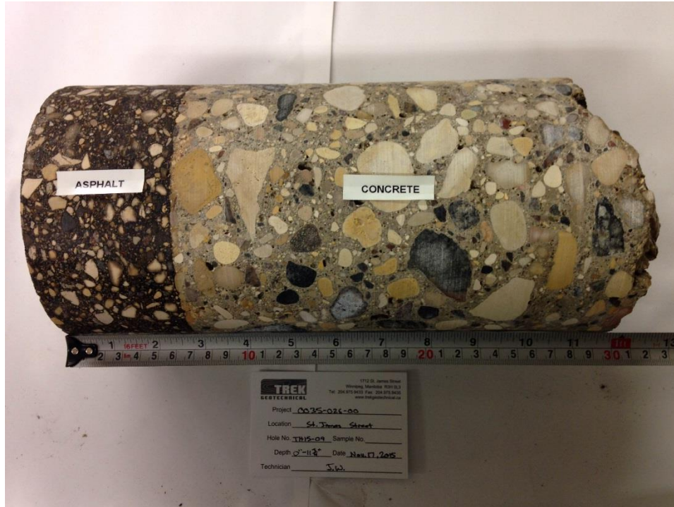
Photo 9: Concrete Core Sample From Test Hole TH15-09
