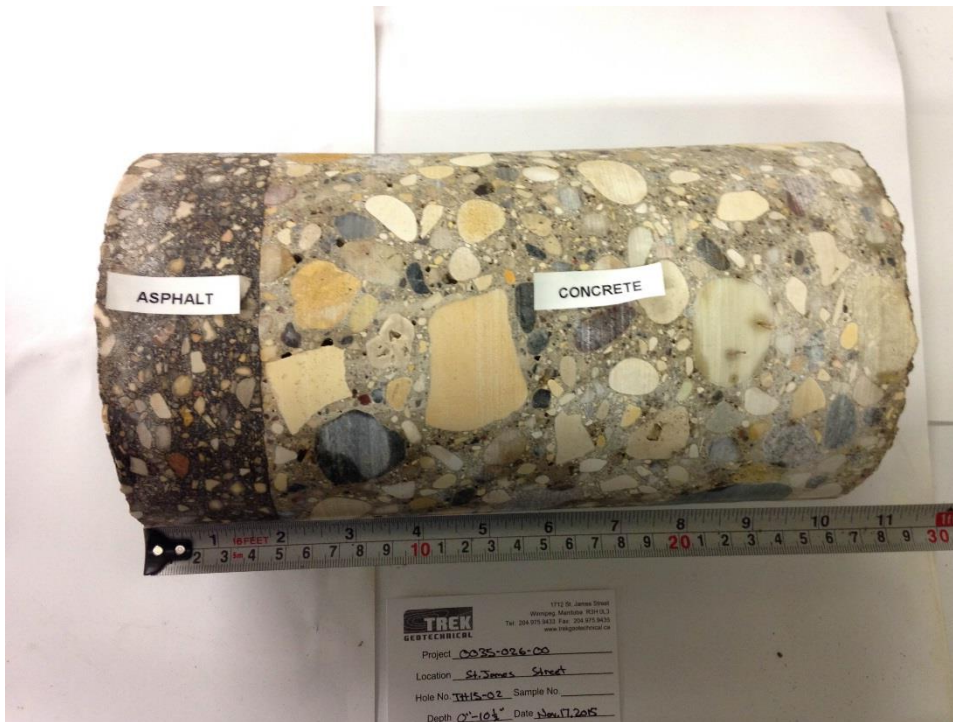
Photo 2: Concrete Core Sample From Test Hole TH15-02
