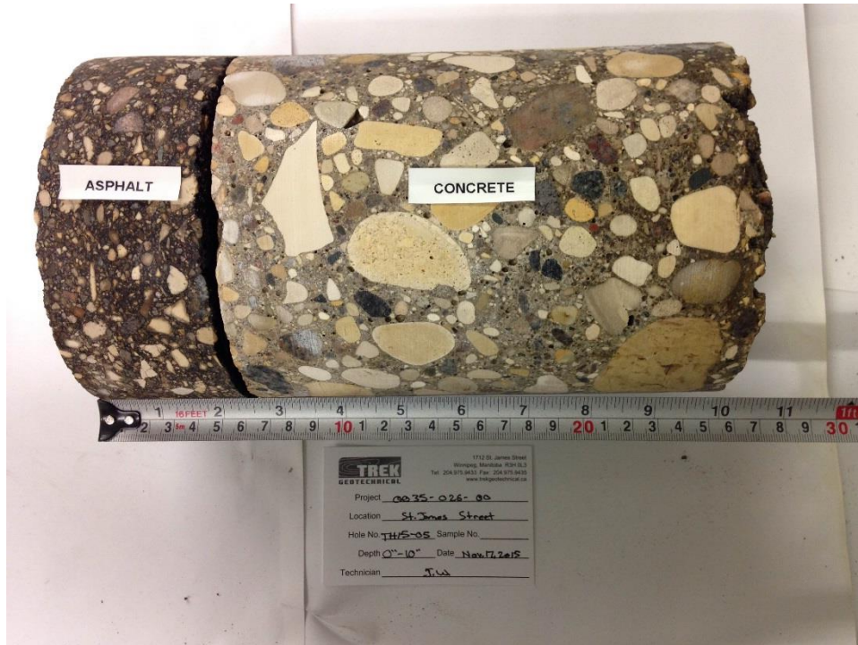
Photo 5: Concrete Core Sample From Test Hole TH15-05
