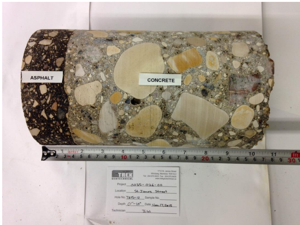
Photo 12: Concrete Core Sample From Test Hole TH15-12
