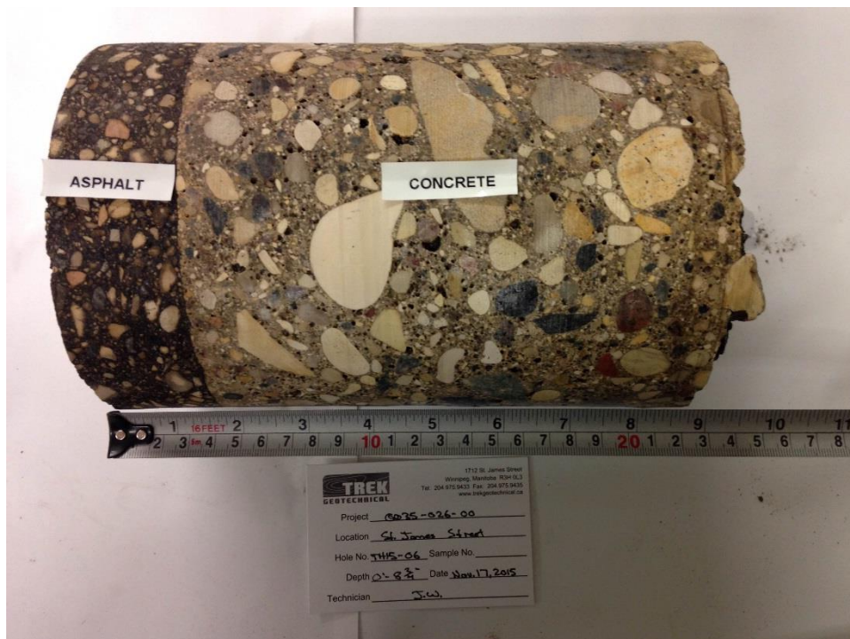
Photo 6: Concrete Core Sample From Test Hole TH15-06
