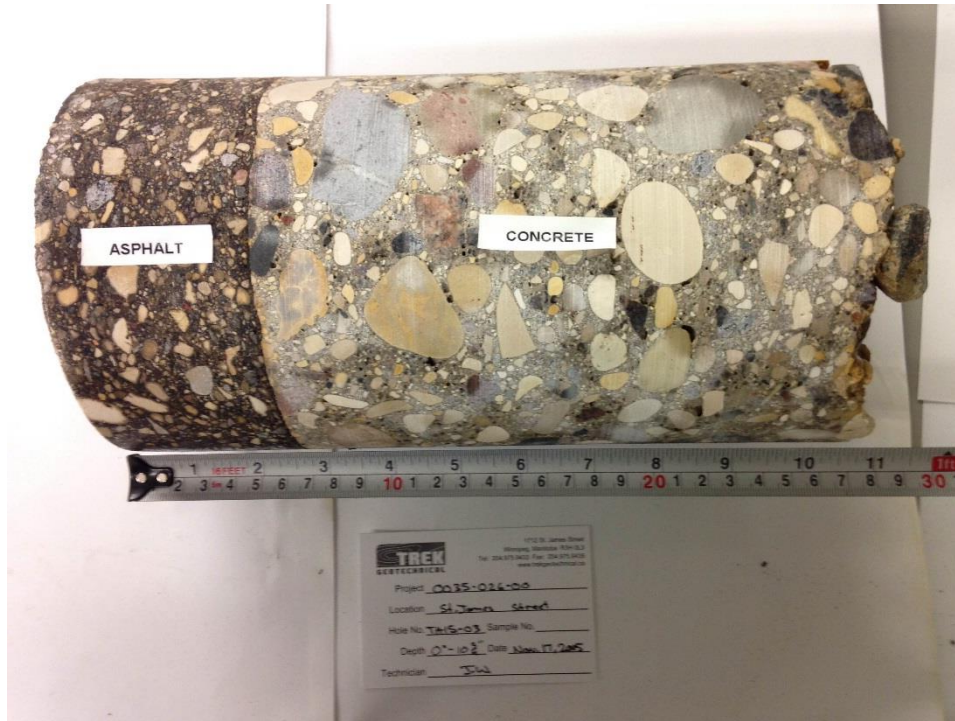
Photo 3: Concrete Core Sample From Test Hole TH15-03
