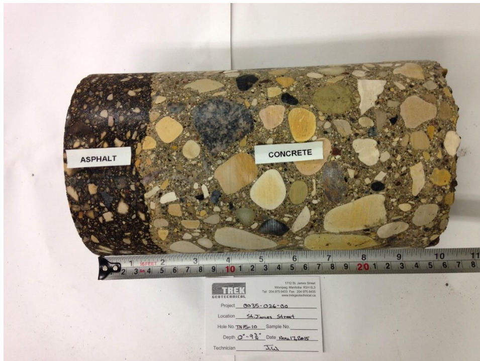
Photo 10: Concrete Core Sample From Test Hole TH15-10
