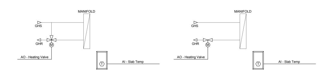
IN-FLOOR HEAT SCHEMATIC SCALE: N.T.S.
