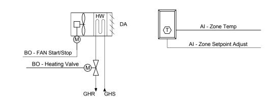
UNIT HEATER SCHEMATIC SCALE: N.T.S.
