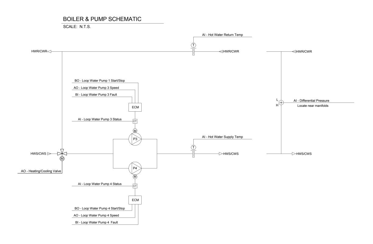
HEATING SYSTEM SCHEMATIC SCALE: N.T.S.
