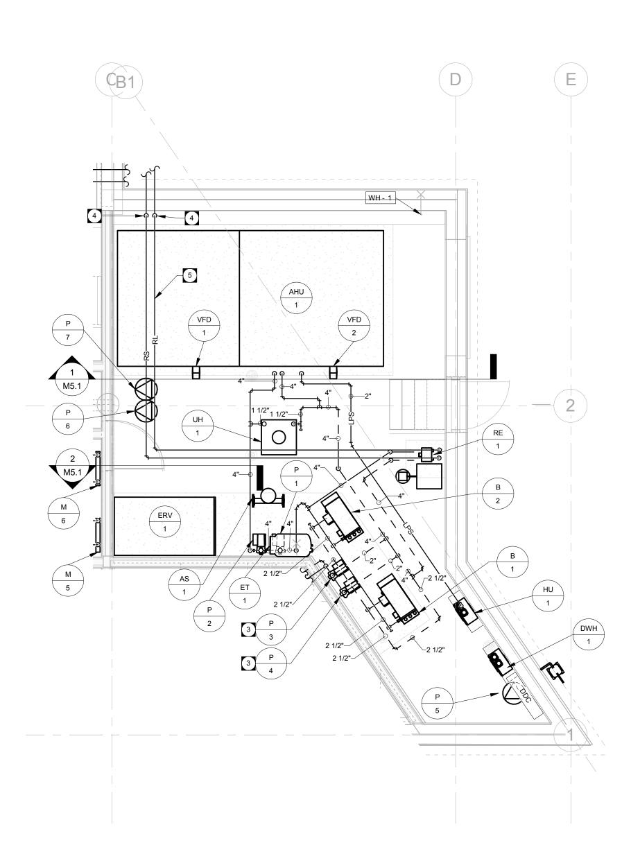
LARGE SCALE PLAN - MAIN HYDRONIC SCALE: 1/4" = 1'-0"
