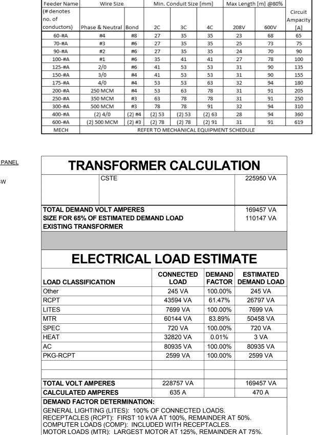
HEATING OR AIR COND (HEAT OR AC): LARGEST TOTAL OF HEAT OR AC. SPECIFIC LOADS (SPEC): LARGEST AT 100%, REMAINDER AT 100%.
