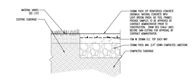
COMPACTED AGGREGATE SURFACING, TYP.
