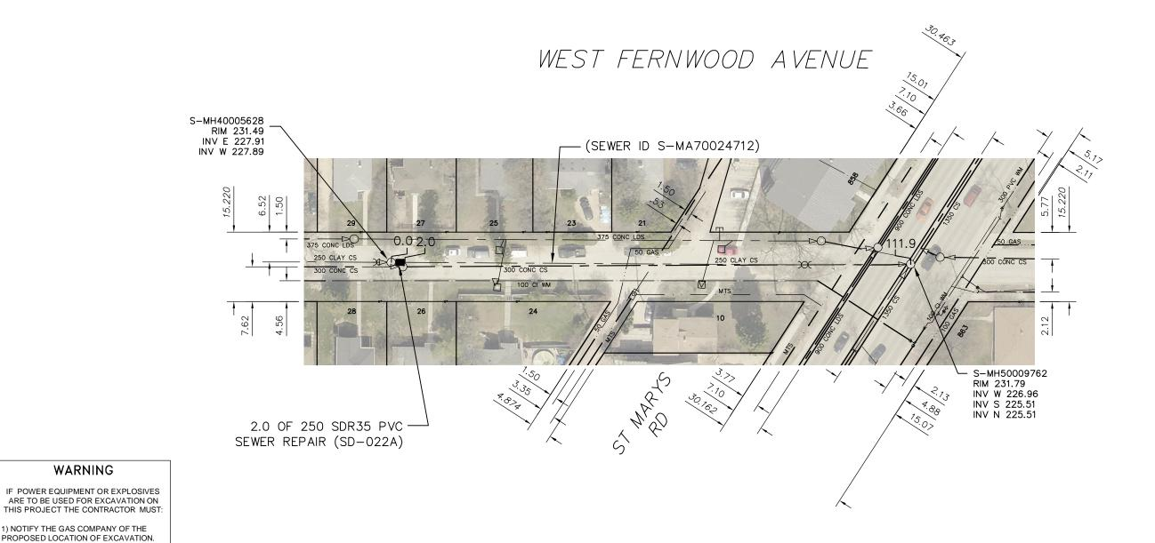
SEWER JUNCTION INFORMATION FROM SEWER VIDEO INSPECTION SEWER ID S-MA70024712 DISTANCE FROM MH ID S-MH50009762 DISTANCE DIAMETER CLOCK 10.1 10 11.0 150 25.8 150 26.6 150 10 43.7 100 10 49.8 150 57.7 150 10 58.0 150 10 91.4 100
